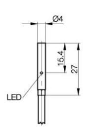
**Inductive Sensors** BES 516-3008-G-E4-C-PU-02 D4 x 27 normally-open Sn=1,5mm shielded
